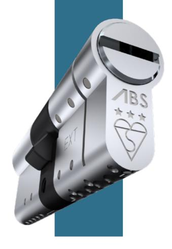
A sacrificial cut is used so that when the burglar grabs the end of the cylinder, just the tip snaps off, leaving more metal in front of the central locking mechanism as protection.
